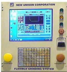
The 1500 is equipped with highly reliable AC Digital Servo Motors and Drive Amplifiers which are backed a five year warranty from the date they are manufactured by Yaskawa. The Workhead features a high torque 29 Nm direct drive motor to maintain precise work piece positioning during grinding by incorporating a 20 bit high resolution encoder resulting in better part accuracy.
